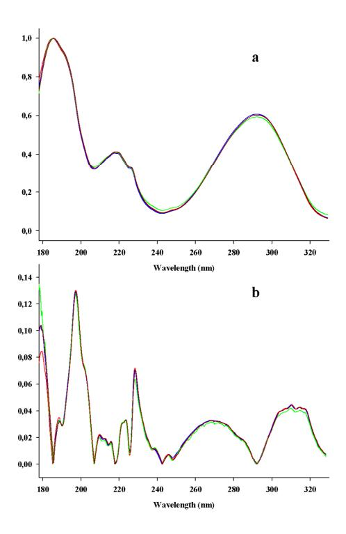
Fig. 1 a/ Overlaid normalized absorption spectra for 4-Nitroaniline recorded during a perio of several years b/ first derivatives with absolute values for the same spectra as in a/
